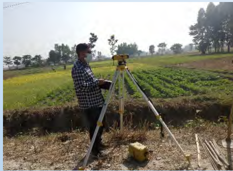
Canal Profile Survey by KIMO and WUA Member with TCP-PIAT Expert (Model Site of S-17, T-2)
